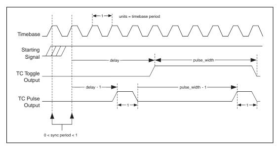
Figure 2-9. Pulse Generation Timing
